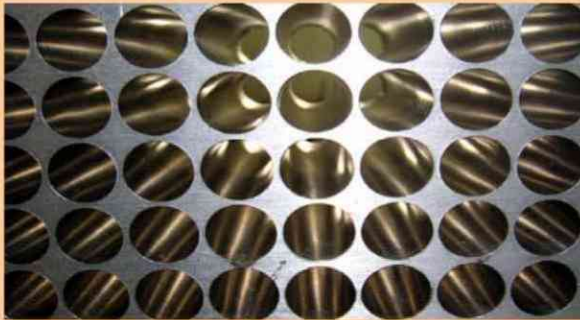
(Hole surface after drilling deep hole 7xD)
